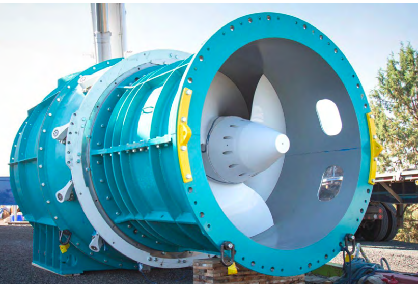
A fish-safe turbine designed by Natel Energy. Courtesy of Natel Energy
