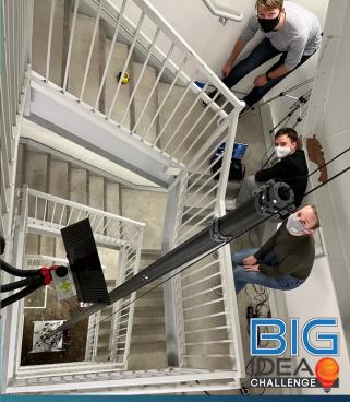
Photogrammetry static deflection experiments at 8.5m and 11m height with MIT's self-deploying lunar tower prototype.
