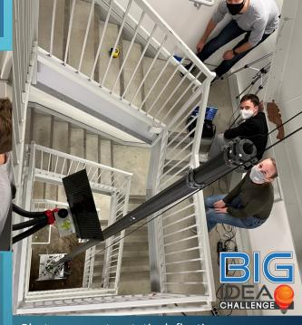
Photogrammetry static deflection experiments at 8.5m and 11m height with MIT's self-deploying lunar tower prototype.
